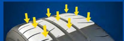
Tire loads cause changes in both tread temperature and wear
